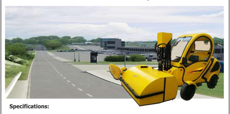
Sweeping width Max (MM) :1650 Sweeping width Min (MM) :1250 Waste container capacity (Ltrs):415 Trailer capacity (Gross KG) :700 Area coverage (~ Sq.Mtr.) : 16,000 Gradability (Degrees) :35 Working speed range (KMPH) :5 to 12 Machine weight (KG) ~ :1595 Dimensions (L\*B\*H) in Mtr :3.6\*1.8\*2 Hopper lift height (MM) :1200
